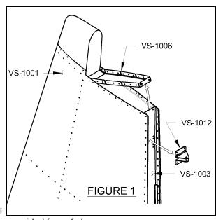
REQUIRED ACTION To satisfy this Service Bulletin, install a hinge doubler as detailed below. The hinge doubler will be provided free of charge.
